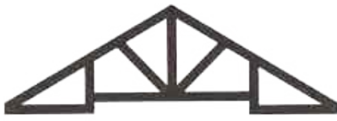
09. King Post Truss with Straight Diagonals
