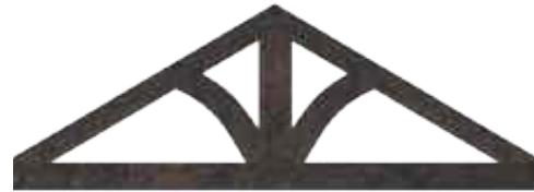
02. King Post Truss with Arched Diagonals
