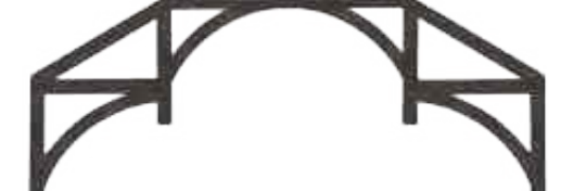
12. Hammer Beam Truss with Rafter Tails
