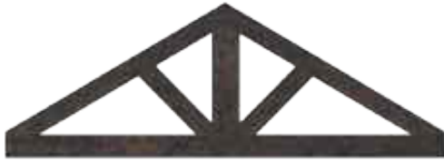
01. King Post Truss with Straight Diagonals
